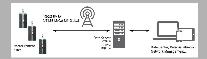
Data is transmitted efficiently in real time from your monitoring well to your mobile phone or computer. Transmissions can occur via HTTP(S), MQTT(S), and FTP(S).
