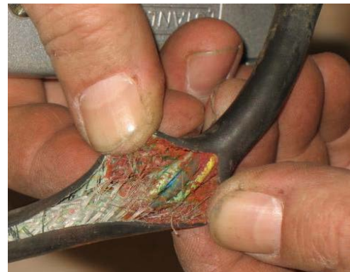
Figure 3. Do not use Zip-Ties Directly on Cables
