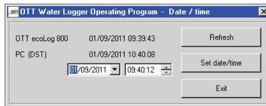
Fig. 25: Setting the OTT ecoLog 800 (3G) date and time.
