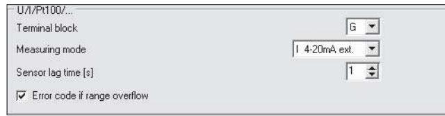
Fig. 15: Setting operating parameters of the OTT netDL function block I 4-20 mA .
