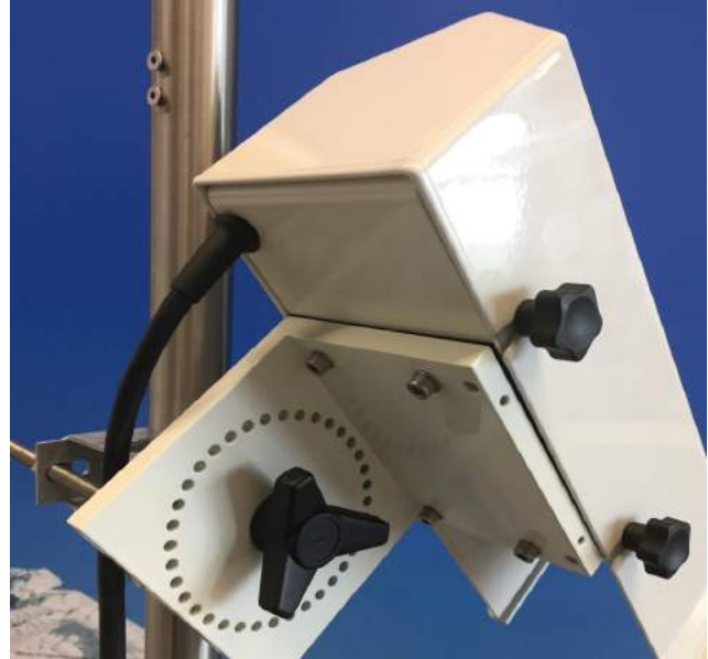
Figure 14: Sensor mounted with hood. After the cable has been installed, the weather protection hood is fixed again over the 3 knurled screws.
