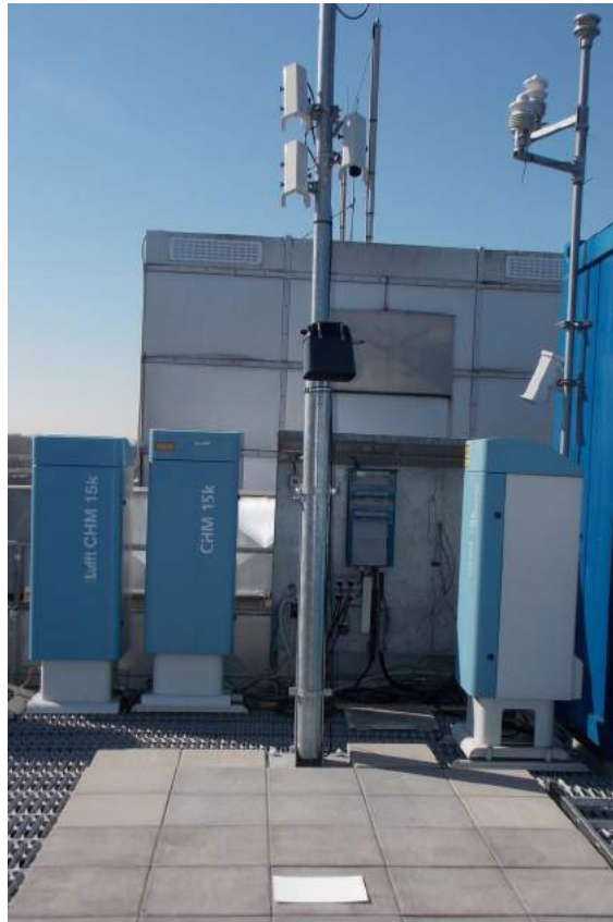
Figure 31: Check of the signal quality using the white board 8365.KWK-WS
