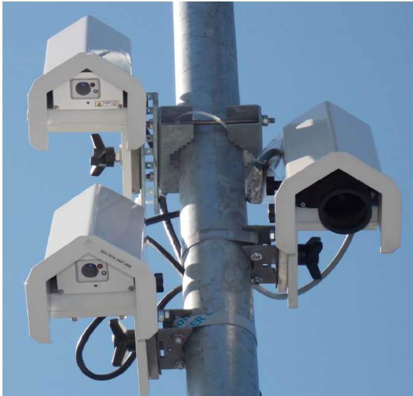
Figure 12: SHM 31 sensors with mounting clamp 8365.610-11 (upper left), mounting clamp 8365.608-11 (lower left) and a SHM 30 Sensor with mounting clamp 8365.608-11 (middle right).
